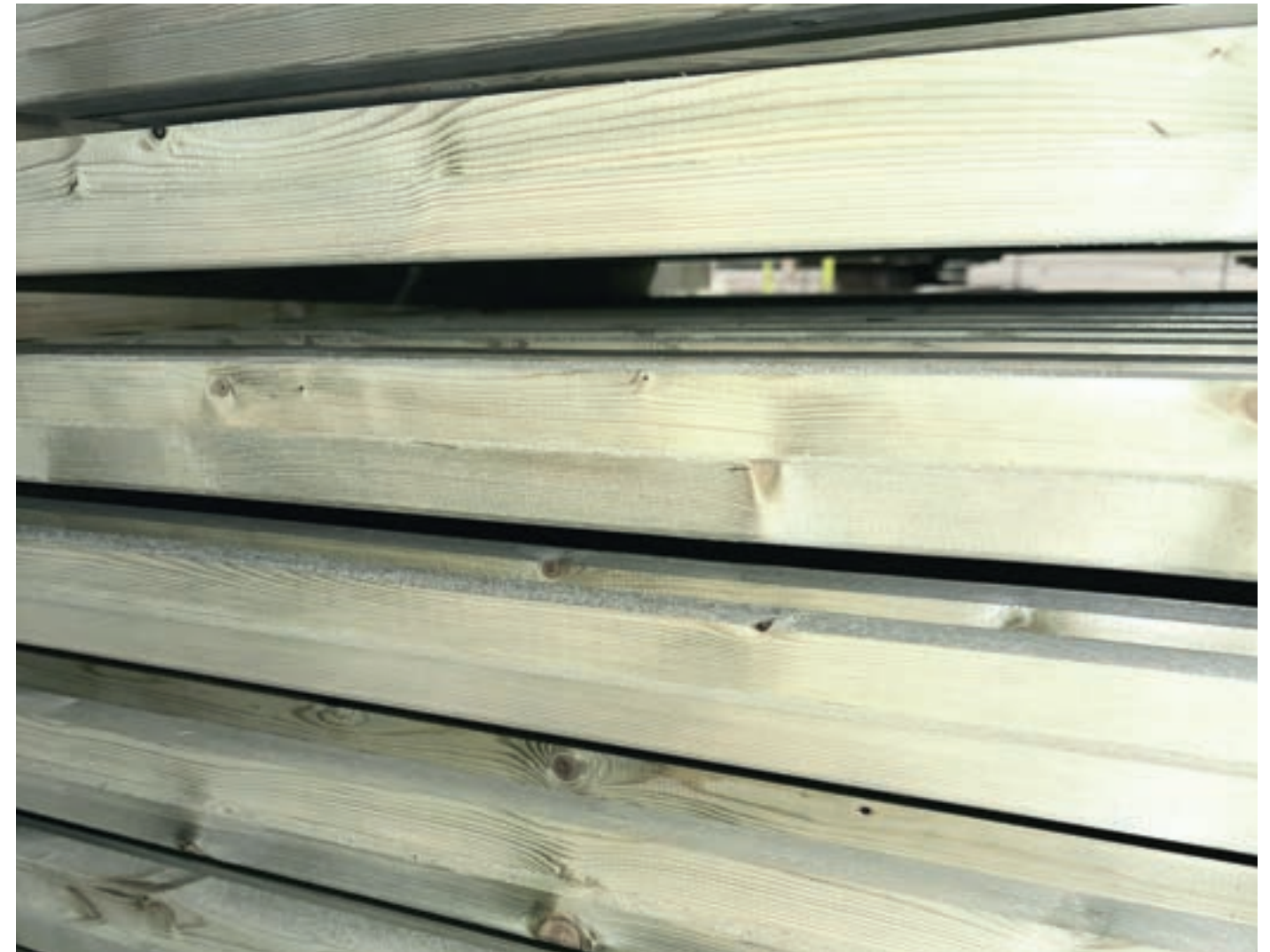
Latted timber drying process
